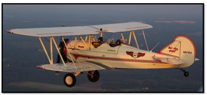
**Takeoff:** Takeoff happens sooner than one might expect, especially if anticipating Stearman-like performance as I was. Four Piper Cub-series wings on the same aircraft mean a lot of lift is being generated! By the time there is enough speed to raise the tail, the high-camber wings are ready to climb, whether you apply backstick pressure or not. Takeoff will occur in 600 feet or less. Climb-out at about 65 mph will yield a 600-700 fpm climb rate.
